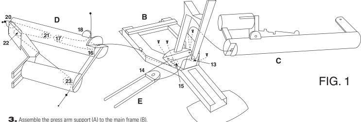
**3.** Assemble the press arm support (A) to the main frame (3/8-16 x 1/2 hex screws, qty. 4). **FIG. 1**.
