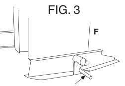
Spring loaded positioning pin shown in latched position
