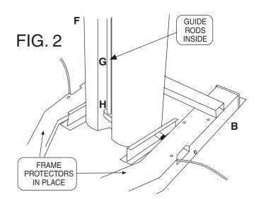
frame protectors in place throughout this step. **FIG. 2.** The positioning pins have to rise and snap into the notches provided at the base of the stack column (F). Because the springs holding down the pins are stiff, a fair amount of force is required. For the last two inches, tilting the stack column (F) toward the press arm support (A) helps by making the ramps less steep.
