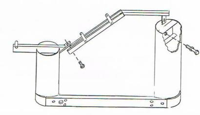
8. Attach cable connection tube to press yoke. (3/8 -16 x 3/4" socket head screw, gty: 2). Do not tighten yet. 9. Attach press yoke assembly to
