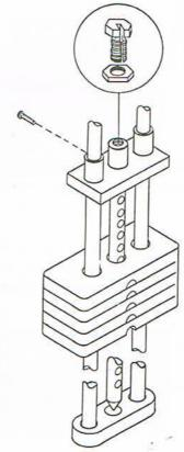
22. Attach the cable to the weight stack. Make sure cable does not twist as you tighten bolt.
