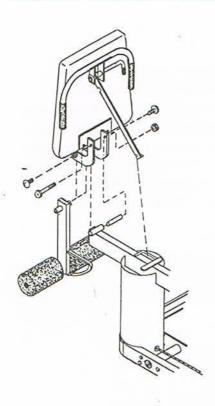
14. Attach the seat bottom assembly using clamp tube and bolt (5/16-18 x 3"). Tighten this bolt very tight. Ensure that the support strut latches at the top of the leg machine column. The strut pivot should be bolted on just tight enough to swing freely.
