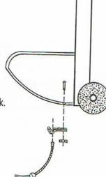
Place the rubber weight stack bumper and guide rods on the weight stack support.
