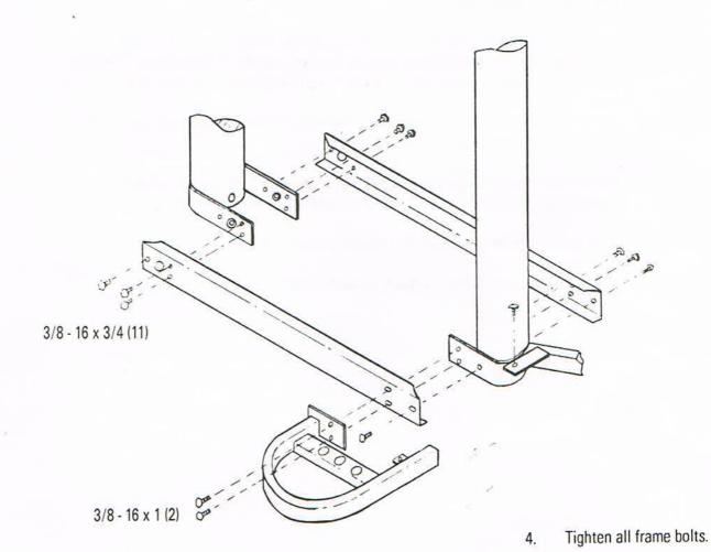
Attach "A" member as shown, tighten bolts very tight.
