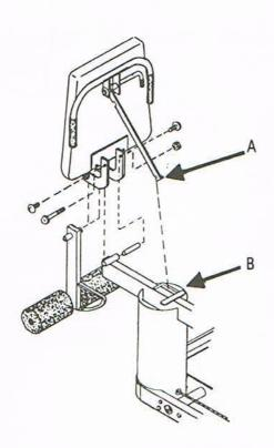
Install leg/ab seat bottom (5/16 – 18 screw, nut and pivot tube).
