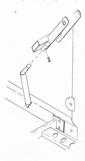
Connect press cable. Secure with 1/4-20 screw and nut.
