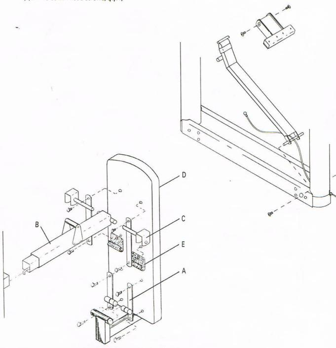
6.a. Attach lower seat pivots (A) to leg station, then to seat back (D).
