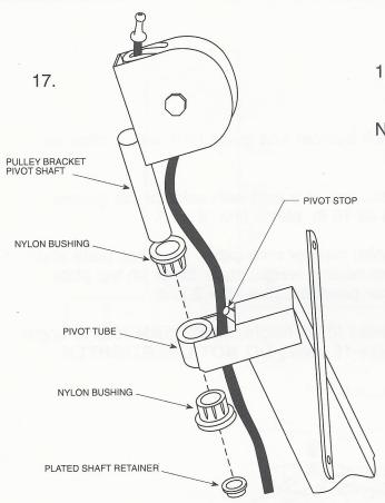
17. Push nylon bushings into pivot tube. Insert pulley bracket pivot shaft through bushings.
