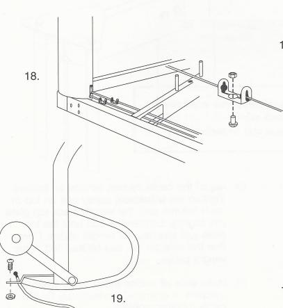
18. Being careful to not lose cable ends into columns, connect leg developer, and abdominal crunch cables to the cables at the base of the main column. Insure that the cables pass through the opening in the weight stack support stringer. Insure that the cables are not crossed.
